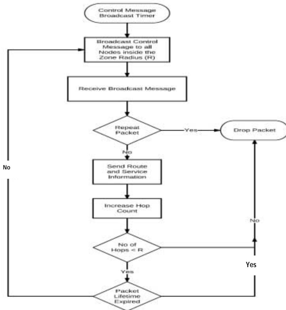
Fig1. Broadcast Mechanism
